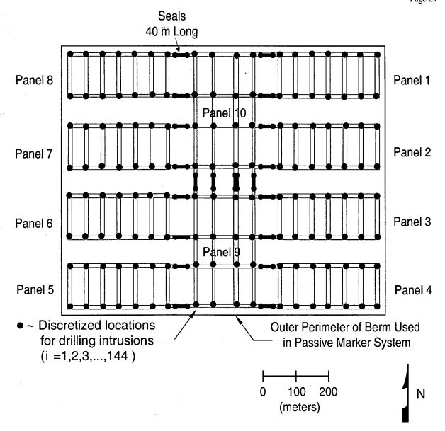
Figure 10. The location of drilling nodes.
