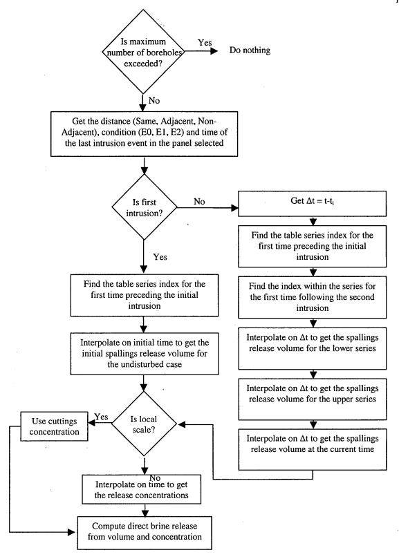
Figure 15. Computation of Spallings Releases.
