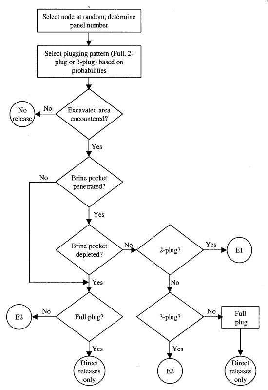
Figure 12. The determination of the type of intrusion.
