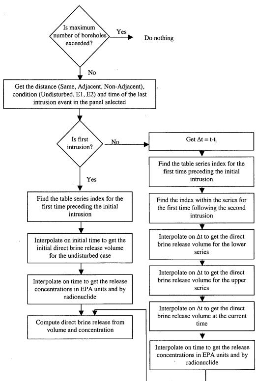
Figure 14. Computatation of Direct Brine Releases.
