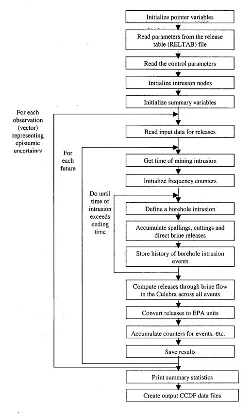
Figure 18. Flow of processing of input data to produce CCDFs.
