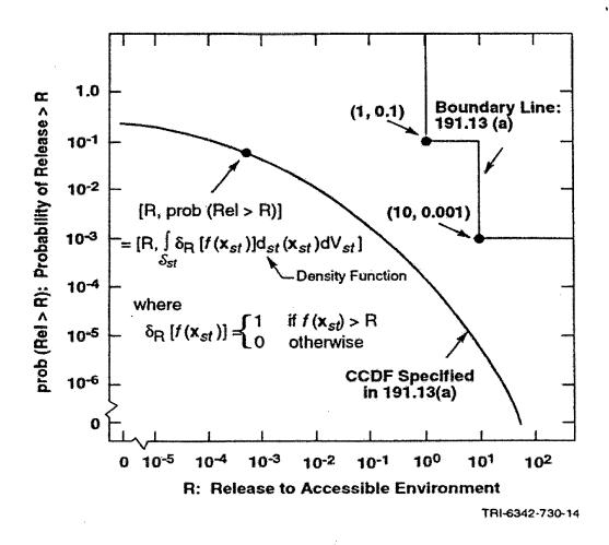
Figure 1. Boundary line and associated CCDF specified in 40 CFR 191, Subpart B.
