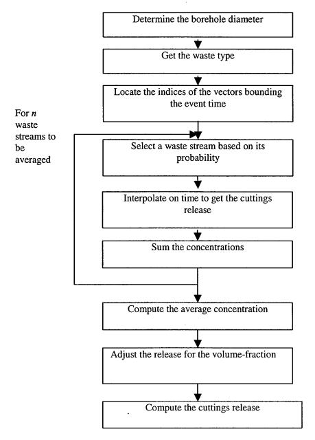
Figure 11. Calculation of Cuttings Releases.
