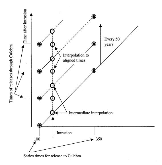
Figure 17. Interpolation for Release to Culebra for a Single Intrusion
